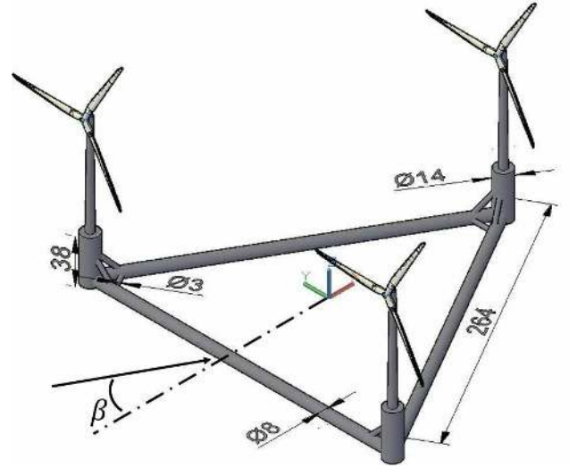
FIGURE 1. The triangular semi-submersible platform. All dimensions are in meters.
