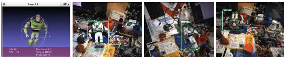
Fig. 1. We show that feature extractor layers from modern object detectors pre-trained on real images can be used on synthetic images to learn to detect objects in real images. The top-left image shows the CAD model we used to learn to detect the object in the three other images.
