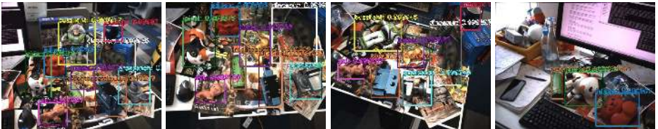
Fig. 12. Results of Faster-RCNN trained on synthetic images only with the feature extractor frozen. The objects are detected in highly cluttered scenes and many different instances are available in one image. Note that the different objects are seen in different arbitrary poses.
