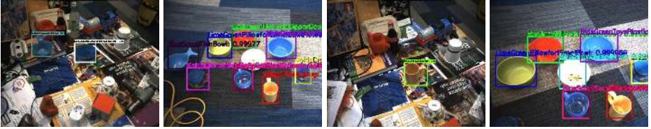
Fig. 14. Objects with similar shapes and colors detected in challenging environments. The detector was trained on synthetic images only.
