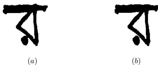
Fig. 3. (a) Ordinary mean filtering joins two disconnected components; (b) Restricted mean filtering does not join originally disconnected components
