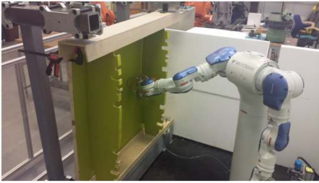
Figure 8. Positioning of the rib by the robot in the physical demonstrator of the test cell
