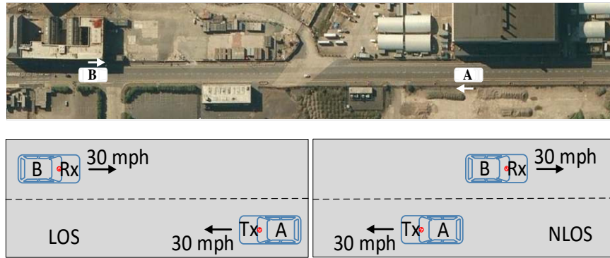
Fig. 8. Satellite view of V2V measurement environment showing the position of two vehicles and two different scenarios (LOS and NLOS channel conditions). It should be noted that the road is approximately 10 m in width.
