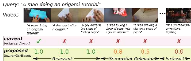
Figure 1: All current video retrieval works treat caption collected for a certain video as relevant, even when other videos are equally relevant to a query text. This makes the evaluation of popular datasets ad hoc at times. We propose to use continuous similarity, allowing multiple videos to be treated as equally relevant. Ex. from MSR-VTT [64].
