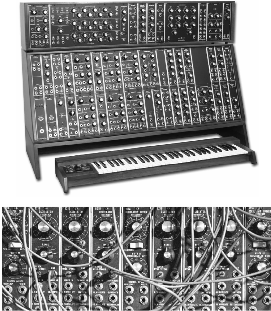
Figure 2 A Robert Moog Studio-66 System modular synthesiser from 1970 (top) and details of a similar model with patch cords applied (below)
