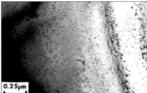
FIG. 5 Interphase precipitation of NbCN in ferrite in steel containing .09%C - .07%Nb. Specimen reheated at 1250°C, rolled at 1000°C, and air cooled to RT. (19)
