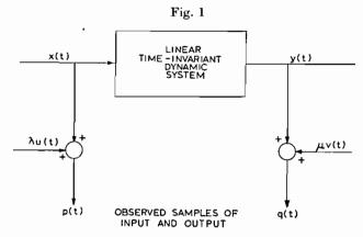
Block diagram illustrating the assumed situation in which system parameter estimation is performed.
