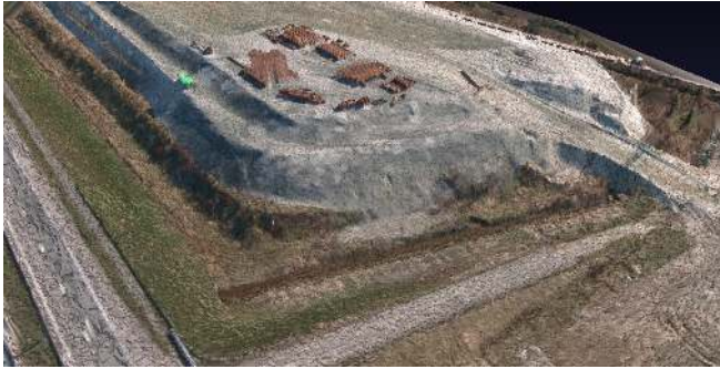
Fig. 4. Close-up of the densely generated 3D model, showing the left side of the hill from figure 2. This visible subsection contains about 1 million vertices.
