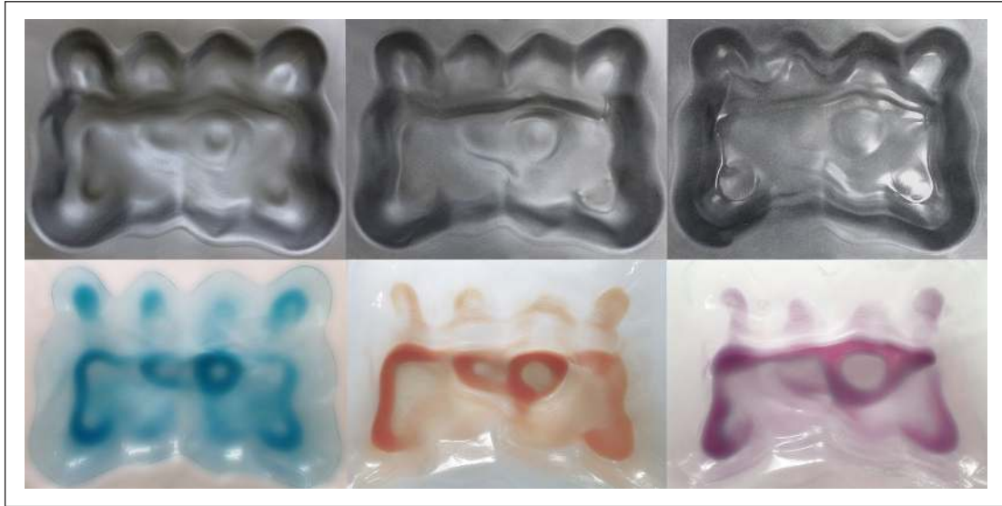
Figure 7. Example of further explorations of computational and material imprecisions in the robotic incremental forming context – manipulation of input geometry allows to generate three different surface compositions from the initial design.
