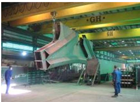
Fig. 1: Handling heavy parts using cranes
