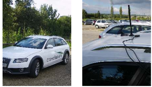
(a) One of the Audi A4 allroad quattro used for measurements (b) Position of the omnidirectional antenna and GPS receiver
