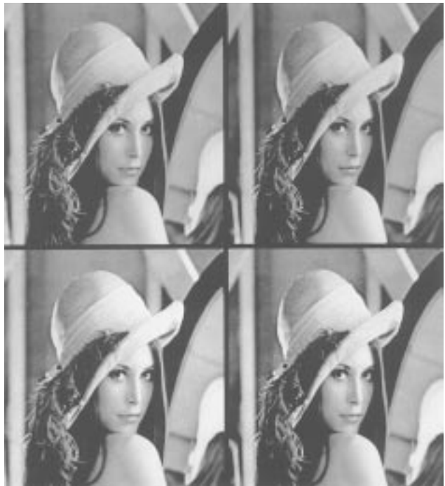
Fig. 16. Monochrome image coded at 8, 0.5, 0.33, and 0.25 b/sample. (The 8-b/sample coded image is at the upper left, the 0.5-b/sample coded image is at the upper right, the 0.33-b/sample coded image is at the lower left, and the 0.25-b/sample coded image is at the lower right.) (From N. S. Jayant et al. , “Image compression based on models of human vision,” in Handbook of Visual Communications , H.-M. Hang and J. W. Woods, Eds. New York: Academic, 1995.)
