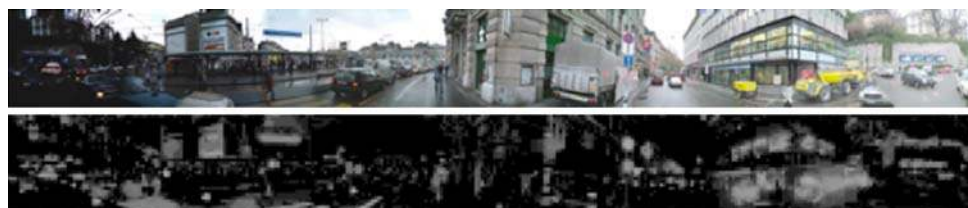
Fig. 4 The picture on top shows a typical urban scene and the picture below shows the corresponding saliency map, as generated by Itti and Koch’s saliency-based model of spatial attention. Each salient or
