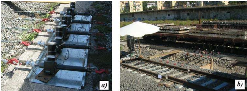
Figure 3. Test system: the series of actuators (a) and the control and acquisition unit (b).
