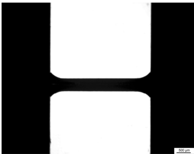
Fig. 3—Transmitted light image of a test specimen with standard geometry.
