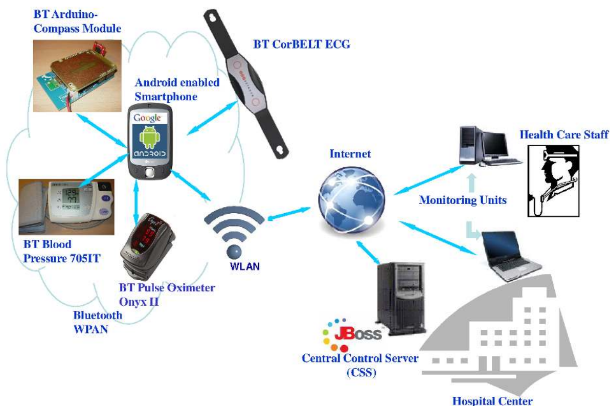
Figure 1. System architecture of the developed prototype.
