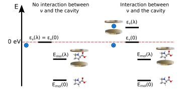
FIG. 2. Pictorial representation of the cavity effect on the energy of the molecule and free electron. If the interaction between the free electron and the cavity is neglected only the energy of the molecular system increases. The energy of the free electron is instead unchanged. On the other hand, if the interaction between the free electron and the cavity is considered, the energy of both the molecule and the free electron increases.
