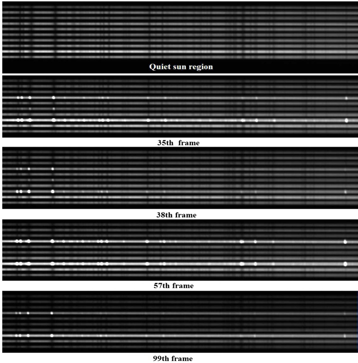
Figure 3. Raw data acquired just before the second contact of the solar eclipse in 2010. The polarimetric pair consisting of the fourth and eighth fiber, counted from the top to bottom in each panel, is used for further reduction. The wavelength increases from left to right and the magnesium triplet are those strong emission lines in the short wavelength region.
