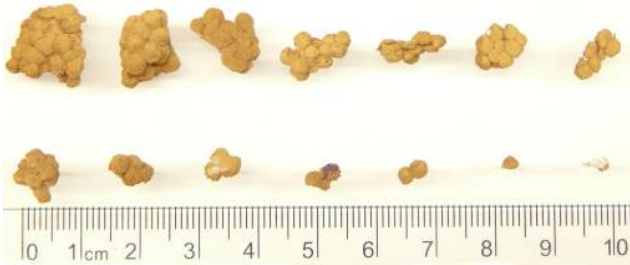
Figure 7. Fourteen Styrofoam particles with maximum dimensions from 2 to 15 mm simulate solid hydrometeors to validate the matching algorithm
