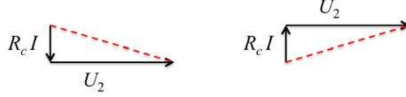
Figure 4. The added orthogonal noise voltages produce the same RMS voltage (and mean-square voltage) even if the sign of the current is flipped to the opposite value. The resulting time-dependent voltages will be completely different however their mean-square (and RMS) amplitude remains the same.
