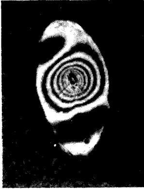
FIGURE 3 Void in the film as viewed with reflected light. Typical void densities are \sim 25 to 100 \text{ cm}^{-2} .
