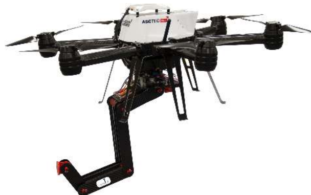
Fig. 1. The Compact AeRial MANipulator (CARMA) mounted on the ASCTEC NEO platform [8].
