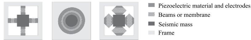
Figure 1. Top view of the different MEMS piezoelectric accelerometers analyzed: trampoline (left), annular (middle) and hexagonal beams with square seismic mass (right).
