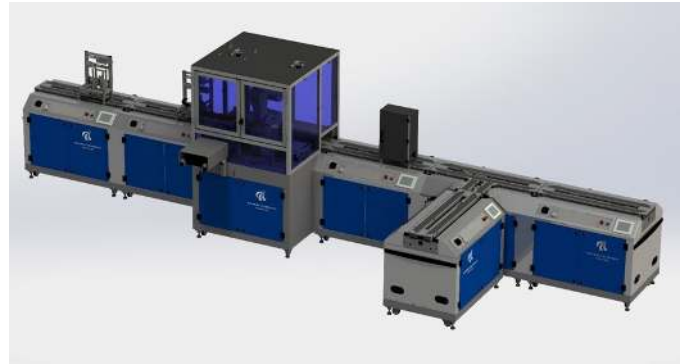
Fig. 1. Reference layout of the production line at the AAU Smart Production Lab composed of 7 interconnected modules. This number of modules translates into 14 process-specific stations as each module integrates 2 stations (one at each of the sides).
