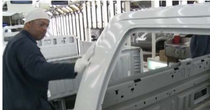
Figure 1: Check-men working on a production line, inspecting car body parts following the painting stage (image courtesy of FORD Dearborn, USA).
