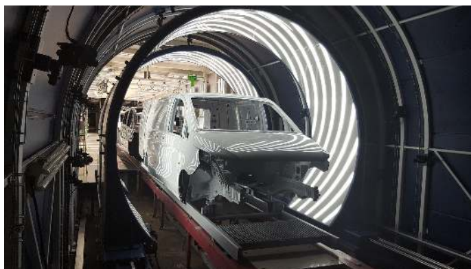
Figure 11: QEyeTunnel: an automated inspection system for car body surface quality control based on artificial vision.
