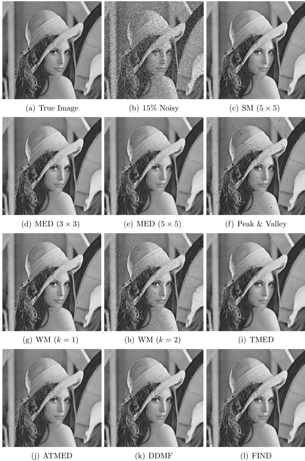
Figure 2.8: Impulsive Noise filtering of Lena image corrupted with 20% of SPN by different filters
