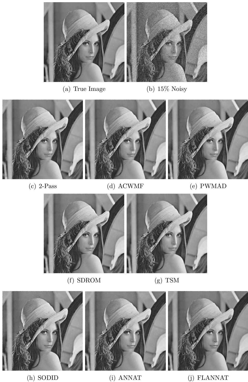
Figure 3.8: Impulsive Noise filtering of Lena image corrupted with 15% of RVIN by different adaptive threshold schemes
