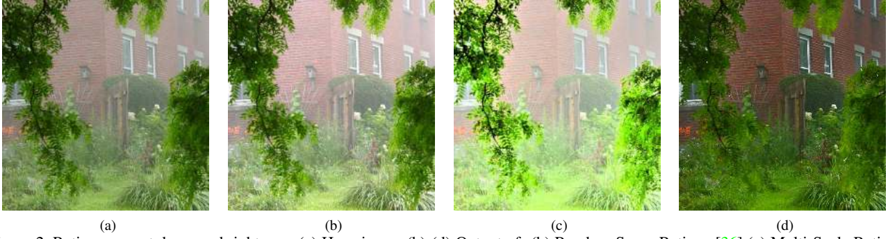
Figure 2. Retinex cannot decrease brightness. (a) Hazy image (b)-(d) Output of: (b) Random Spray Retinex [36] (c) Multi-Scale Retinex [18] (d) Multi-Scale Retinex used for image dehazing, following eq. (1).
