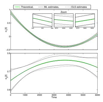
Figure 1: FS-TAR(2) experiment: The theoretical, MLestimated, and OLLS-estimated AR parameter trajectories (mean estimates  $\pm$  two standard deviations; 500 runs).
