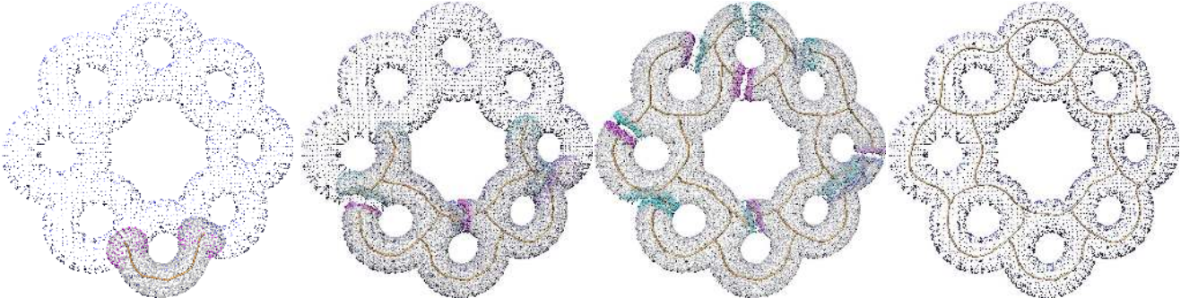
Figure 3: Tracking the center of fronts during reconstruction defines the inner curve-skeleton of a multi-torus object. The topological events on the deformable model are mapped as loops in the curve-skeleton.
