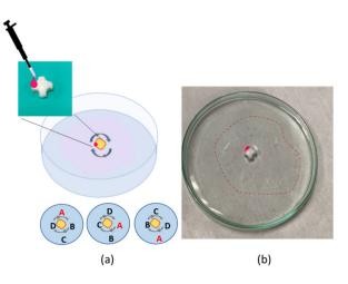
**Figure 4.** (a) Outline of the experiment: the white magnet commonly used for stirring is activated by the dispensing of polymer droplet, and the rotation of the magnet induces the film formation. (b) The polymeric film formed on the fly is indicated by the dotted line.
