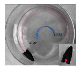
**Figure 6.** The dispensing of the polymeric droplet over the black boat floating on water induces the propulsion along the wall of the Becker and the simultaneous formation of a very thin semi-circular polymeric layer. On-the-fly formed polymer film is indicated by the dotted line.
