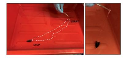
**Figure 7.** When the boat is free to move over a bigger surface, we observed the propulsion from one side to the opposite one. On-the-fly formed polymer film is indicated by the dotted line. The recovered polymeric film attached to the back of the boat is visible.
