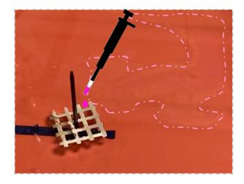
**Figure 5.** Al square grid forms an extended polymeric layer; the expanded film stops the grid's rotation. On-the-fly formed polymeric film is indicated by the dotted line.
