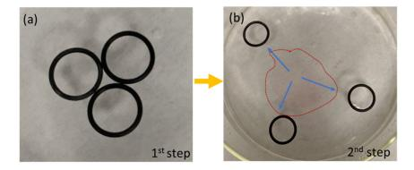
**Figure 10.** (a) Polymer droplets are dispensed in the central area, delimited by the points of contact of the three black o-rings; (b) the instantaneous formation of the film moves the floating objects away, inducing propulsion of multiple objects at the same time. On-the-fly formed polymer film is indicated by the dotted line.
