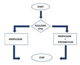
**Figure 1.** Flow chart of the process related to on-the-fly formation of polymeric thin films at water surface.
