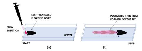
**Figure 3.** Scheme illustrating the mechanism of self-propulsion by the solute capillary Marangoni flow. (a) Dispensing of the polymeric solution for propelling the object (a black boat). (b) Propulsion of the object and simultaneous formation of a polymeric film along the direction of the propulsion. The object while moving over the water surface activates the formation of a thin film by polymer spreading on the water surface.
