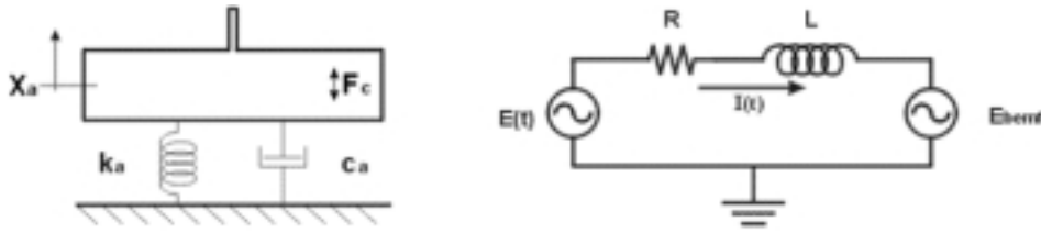
Fig. 3. Exciter's electromechanical model.
