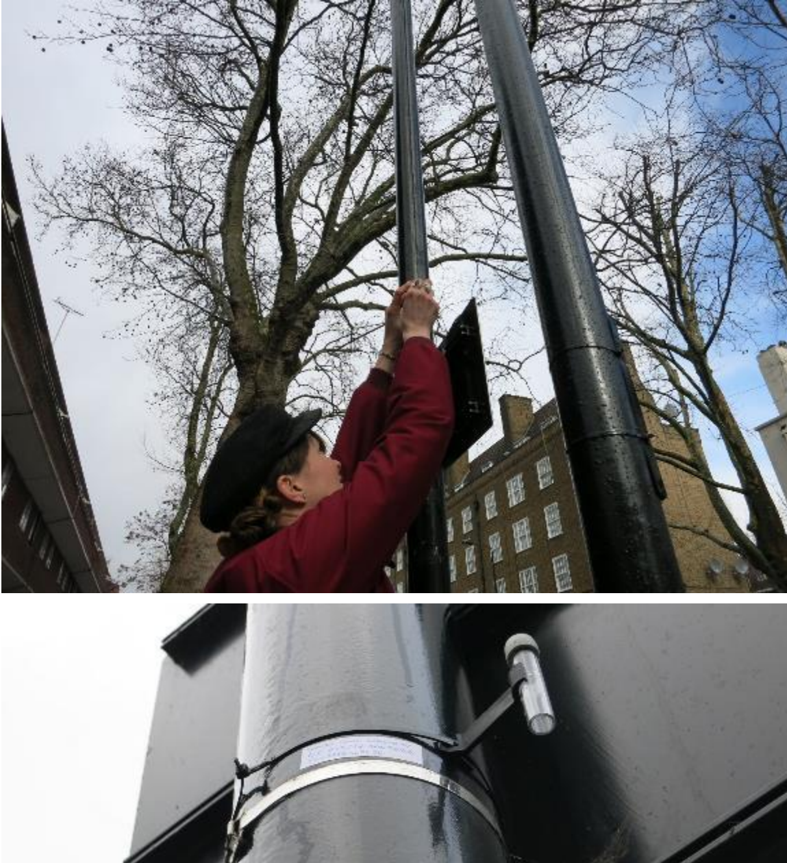
Figure 3 – Installing a diffusion tube in Somers Town and leaving a note about the activity.
