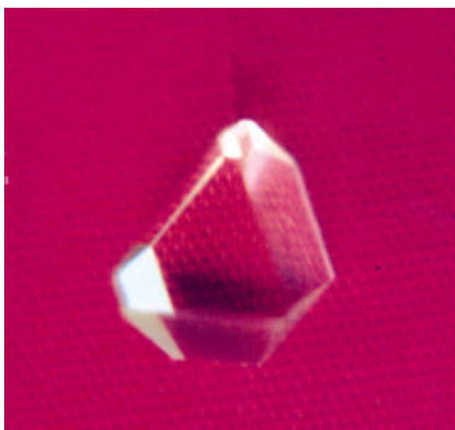
Figure 2. Photograph showing the absence of growth veils in the grown crystals.
