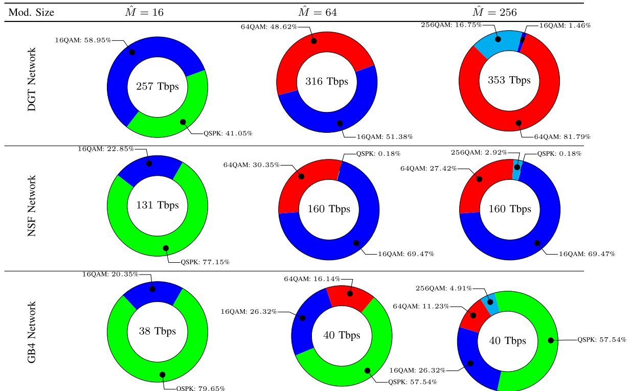
Fig. 13. Percentage of transceivers using different modulation formats for the optimal HD-FEC solution (for 1R_c VarM) and the three network topologies. The results are shown for different maximum constellation sizes \hat{M} .
