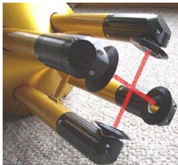
Fig. 1. 2D-S probe. The saucers on the detector arms are designed to minimize shattering fragments from entering the sample volume, which is near the middle of the path between the detector arms for small crystals. However, shattering fragments do still reach the sample volume and are apparent as clusters of small particles with very small inter-arrival times. These artifacts are removed using a detailed statistical analysis, as described by Baker et al. (2009) for the case of splashing raindrops. See text for details.
