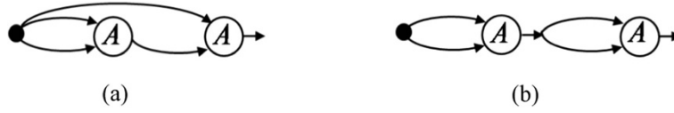
Figure 3 The two graphs with p = 2 A -operations: (a) additive graph and (b) multiplicative graph.
