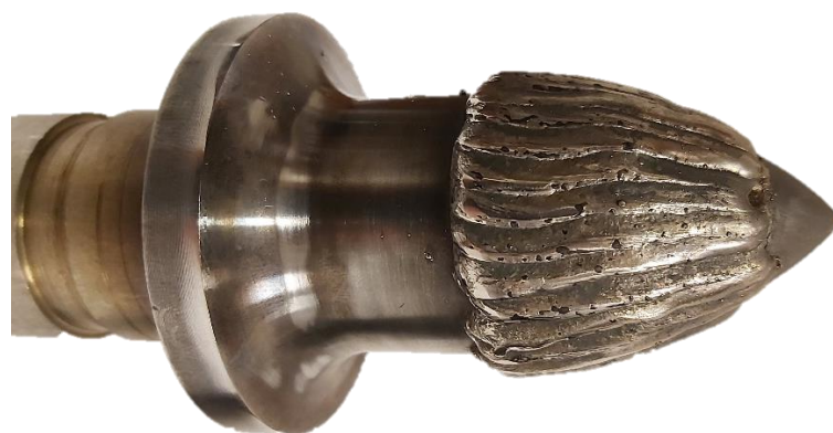
Figure 2. Hard coating applied with robotized GMAW process on the working surface of conical pick.
