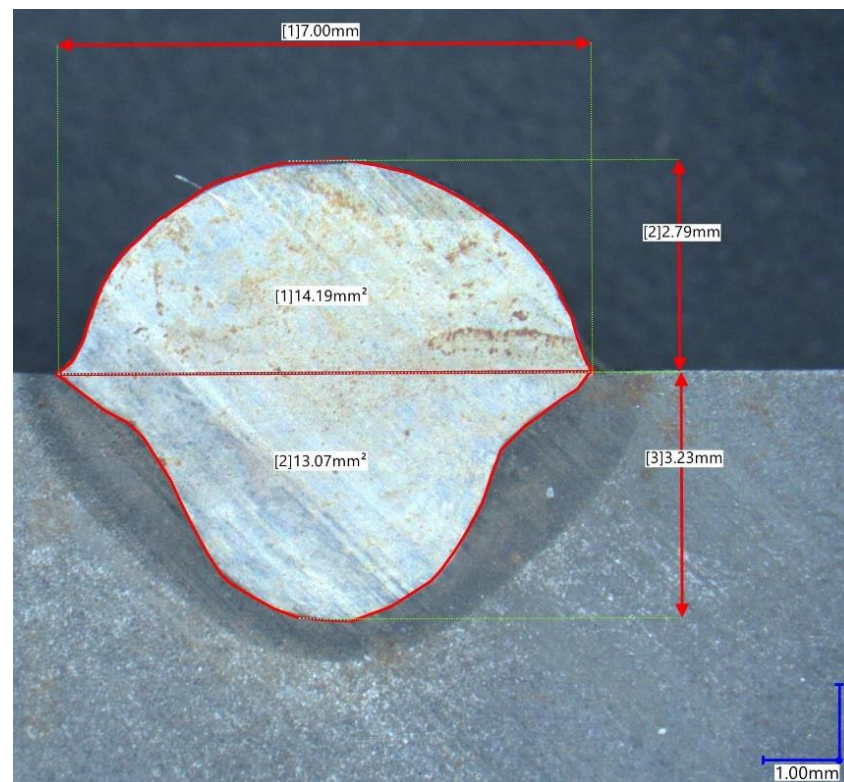
Figure 5. A microscopic view on the cross-sectional geometry of the weld bead.
