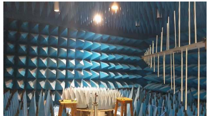
Fig. 2. Tests on the effects of the interference in a VLC system in anechoic chamber
