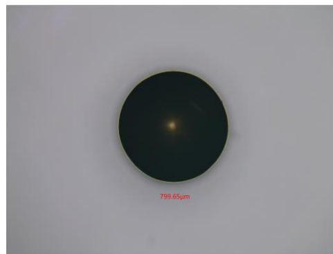
Figure 12. The microphotograph of 800 \mu\text{m} copper particles.
