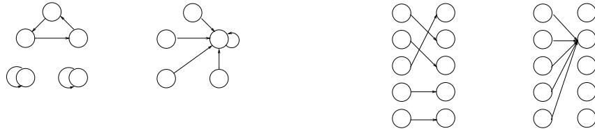
Fig. 2. A permutation and a reset illustrated as transition graphs (left) and as transformations (right).
