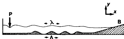
Fig. 1. — Schematic of the experiment. The observation of the amplitude of the wave uses the deflection of an oblique light beam across the water depth. P : vertical plunger ; B : absorbing beach with 12° slope.
