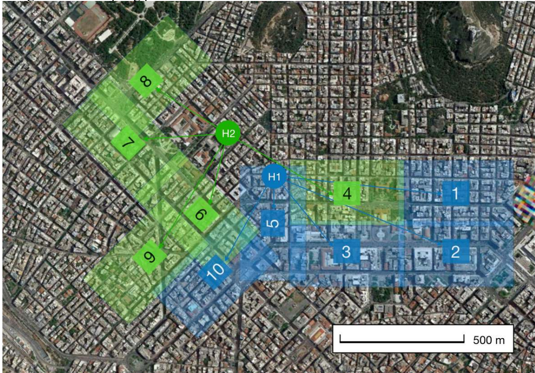
9 10 Figure 3: The route for each drone of the swarm and the two clusters formed
