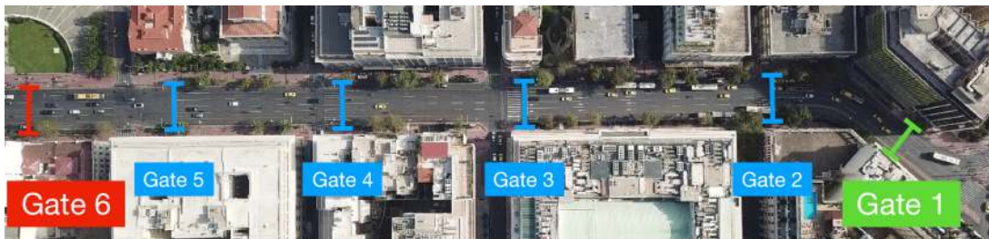
22 23 Figure 9: A main arterial of the study area with installed virtual loops (gates)
