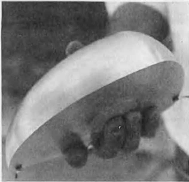
FIG. 3. Photograph of the machined aluminum half-potato that was made by a numerically controlled ball mill and whose ultrasonic resonant frequencies were measured. This object weighs 2438.4 g, and its density is 2.7065 g/cm 3 . Two 1/4 in.-diam transducers cemented to the flat side are visible here.
