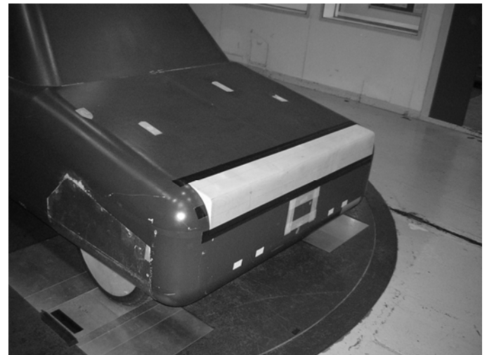
Figure 2 Radius section installed on MIRA full scale reference model
