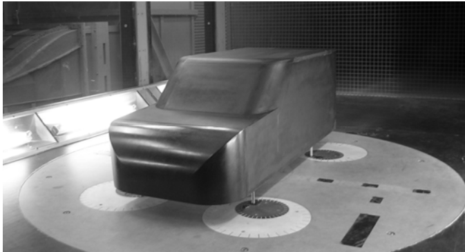
Figure 1 2-box model installed in the Loughborough tunnel
