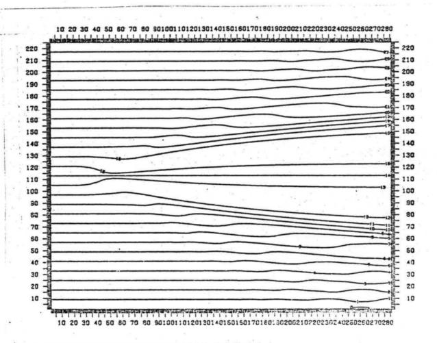
Fig. 4 Energy flux lines for configuration I, according to scheme I  $(\Delta x/L_0 = 1/8)$ .
