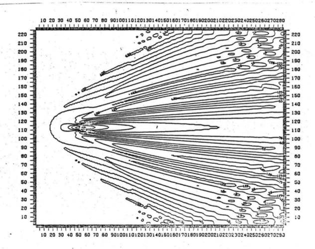
Fig. 2 Contourlines of the amplitude for configuration I, according to scheme I  $(\Delta x/L_0 = 1/8)$ .
