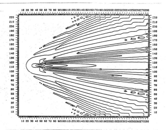
Fig. 3 Contourlines of the amplitude for configuration I, according to scheme II  $(\Delta x/L_0=1/8)$ .
