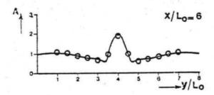
Fig. 1 Comparison of relative wave amplitudes for bottom configuration I, between results of the schemes I and II (continuous curves, Δx/L<sub>0</sub>=1/8) and results of Ito and Tanimoto (1972) and of Flokstra and Berkhoff (1977) (circles).
