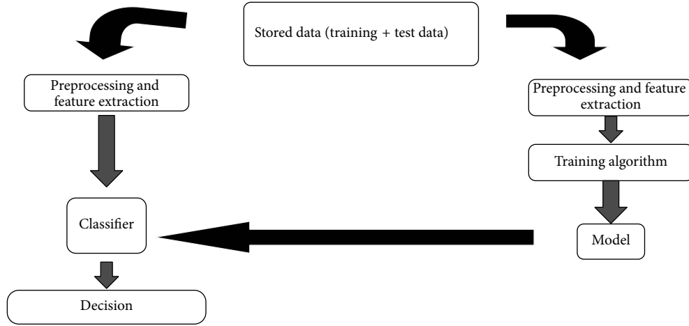
FIGURE 3: Design cycle of handwriting recognition system.
