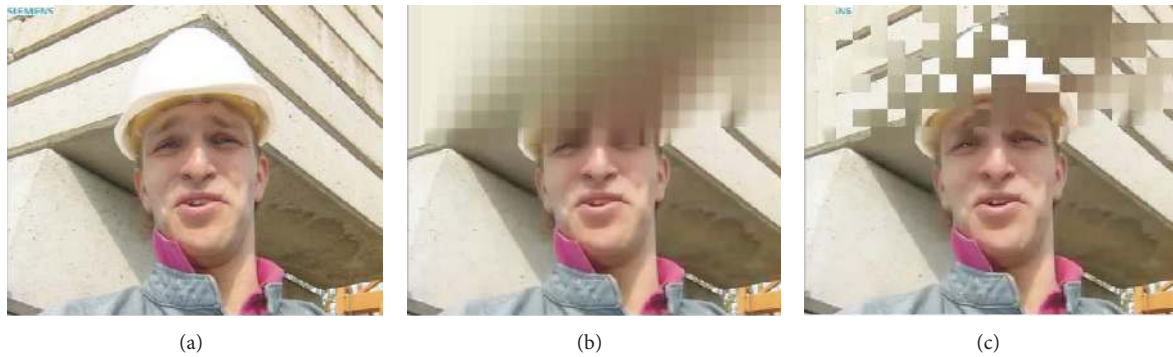
FIGURE 17: Decoded frames between two consecutive bursts: (a) original frame; reconstructed frames (b) 361 and (c) 362.
