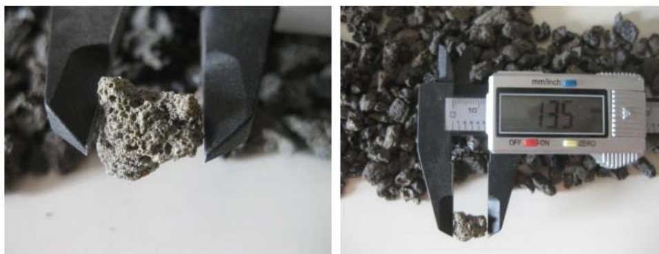
Figure 2. Coarse fraction of the slag produced in the GICC thermal plant and used as recycled aggregate.
